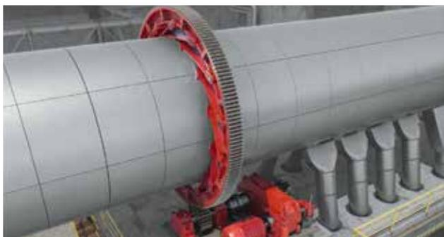
The Segmented Girth Gear (SGG) application installed by SEW-EURODRIVE at the Pellet Plant of Godawari Power & Ispat Ltd. is a mega project that can offer significant new benefits for the steel and cement industries of India. The 14-segment tension spring type SGG, fitted in the Pellet Plant kiln, generates big savings on lubrication (up to Rs. 10 lakh per year), along with reduced maintenance costs and downtime.
