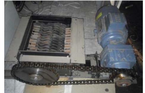
inline type gear motor units were employed. The machines have used R37, R47, R57, R67, R77 and R97 with various motor power and gear ratio combinations.
