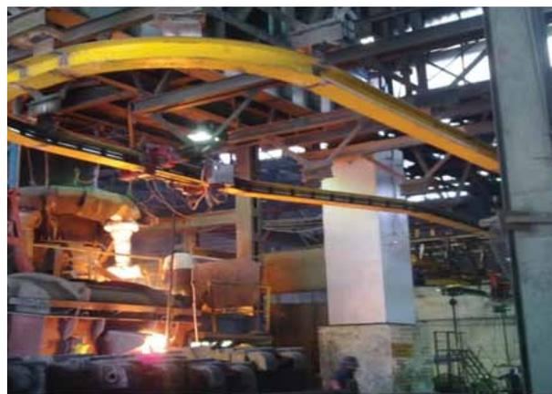
machines. Metal is melted in hot blast cupola of 6T/hr capacity. Dies are then mounted on the rotating carousels and the molten metal is poured. The castings produced are finally annealed, finished, inspected and dispatched to customers.
