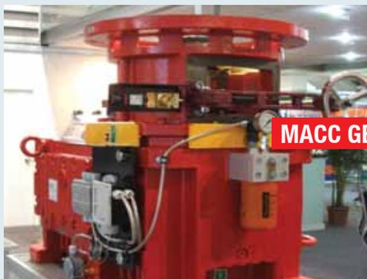
With its wide manufacturing, assembly, sales and service network across the globe, SEW-EURODRIVE presents its dedicated 2-stage Gear Unit Series for Air-Cooled Condensers. These MACC Gearboxes are conceived with design principles based on experience and a well proven existing industrial gear unit series.
